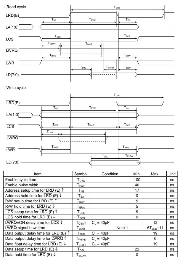
Note 1: When CKSL = Low or CKSL = High, the data output delay time will be  $12 T_{CLK} + 11$ .
