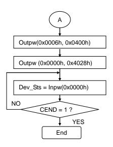
Put a reset instruction command for the " local receive processing complete " flag in the FIFO.
