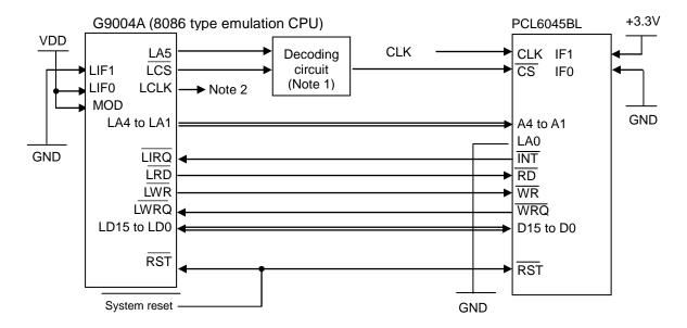
Note 1: The G9004A can be connected to two PCL6045BLs. In this case, the "LA5" signal is used to tell the two chips apart. This line is the equivalent of a decoder circuit. When only one device is connected to the G9004A, there is no need to provide a decoder circuit.
