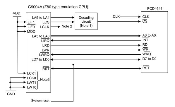
Note 1: When only one device is connected to the G9004A, there is no need for a decoder circuit. The LCS output terminal on the G9004A can be connected to the CS terminal on the PCD4641.
