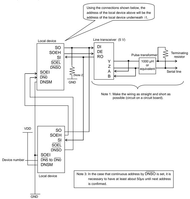
Note 1: When connecting the serial lines to line transceivers, make the path as short and straight as possible.
