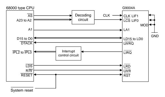
Note 1: Pull the LA5 to LA2, and LA0 input terminals down to GND (5 to 10 K-ohms).
