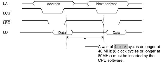
2) Uses the LWRQ output (CPU has a wait function)
