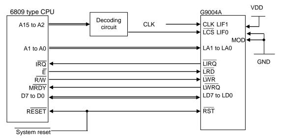
Note 1: Pull the LA5 to LA2 terminals down to the GND (5 to 10 K-ohms).
