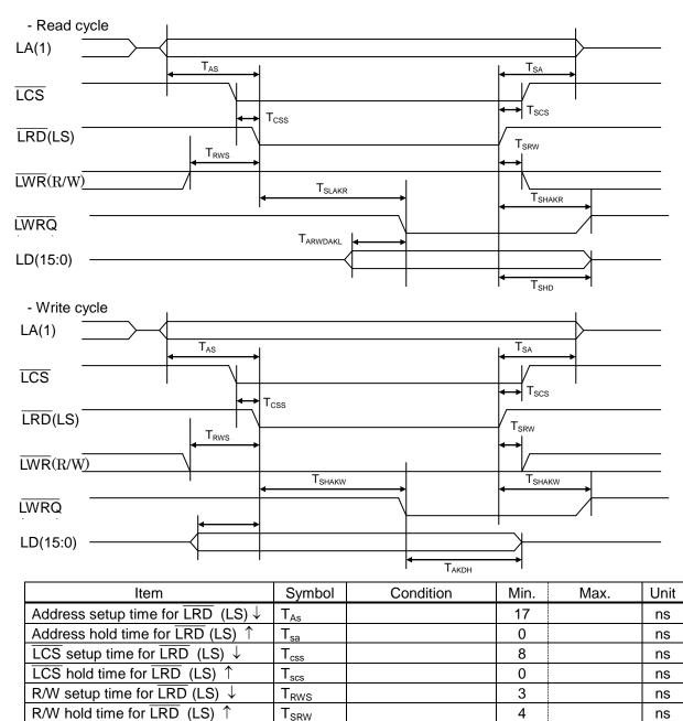
Data hold time for  $\overline{LWRQ}$  (ACK)  $\downarrow$ T<sub>AKDH</sub>0Note 1: When CKSL = Low or CKSL = High, MIN = 4T<sub>CLK</sub> and MAX = 12T<sub>CLK</sub>+9.Note 2: When CKSL = Low or CKSL = High, MIN = 4T<sub>CLK</sub>.
